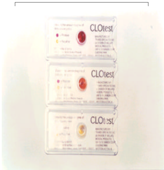
Fig. 1. CLO test kit indicates positive result as red color and negative result as yellow color.
