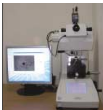
Fig.2. Surface microhardness tester (HMV-2 Shimadzu Co.,Japan) and Polarized light microscope (Axioskop 2 Plus, Zeiss, Germany).
