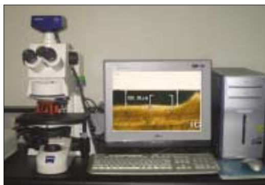
Fig.2. Surface microhardness tester (HMV-2 Shimadzu Co.,Japan) and Polarized light microscope (Axioskop 2 Plus, Zeiss, Germany).
