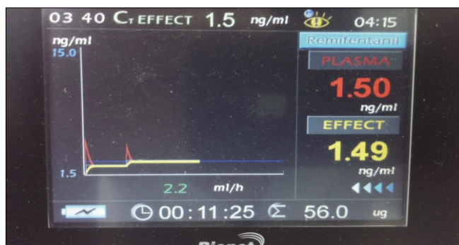
Fig. 5. This display represents plasma and effect site concentration of remifentanyl during anesthesia.
