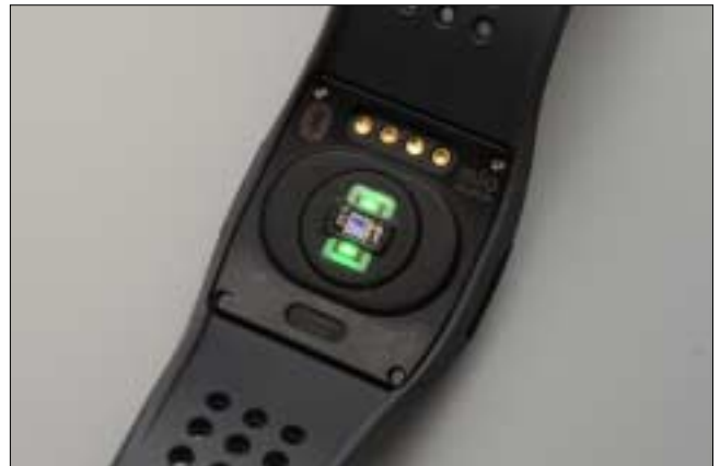
Fig. 2. Back face showing light emitting diode sensors for detecting heart rate.
