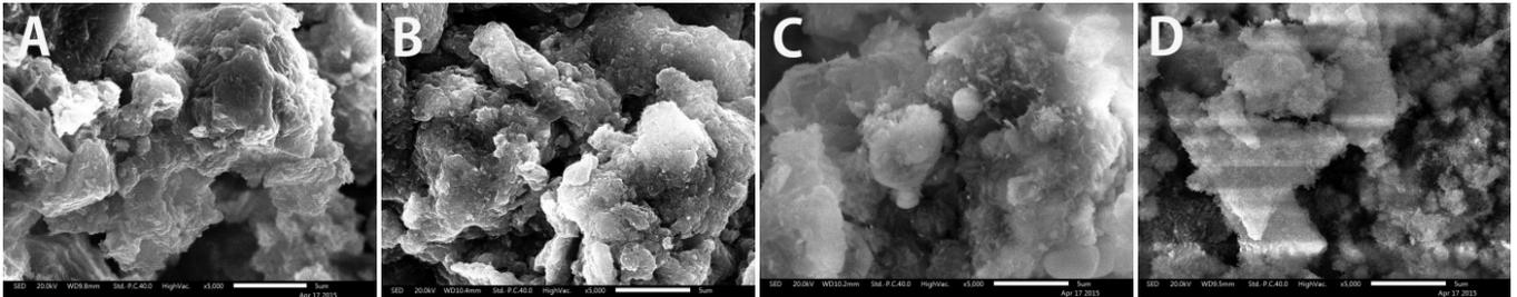
Fig. 2. Scanning electron microscope images of MTA(ProRoot MTA®) exposed to butyric acid at (A) pH 4.4, (B) pH 5.4, (C) pH 6.4 and (D) pH 7.4 after 4-day setting.
