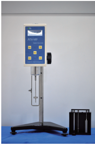
Fig. 1. Viscometer used to measure viscosity in this study.
