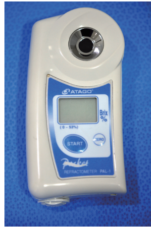
Fig. 2. Refractometer used to measure brix in this study.
