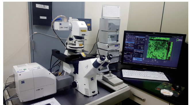
Fig. 4. Confocal laser scanning microscope used to take images of structural form of biofilm in this study.
