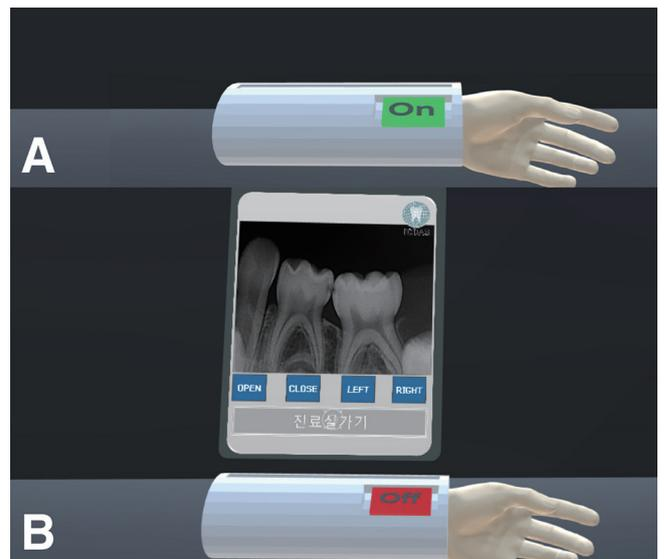
**Fig. 3.** Arm band model with standard x-ray button. (A) X-ray off-states of the arm band, (B) X-ray on-states of the arm band.
