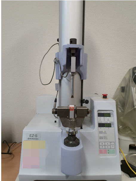
Fig. 3. Universal testing machine for measuring the shear bond strength.
