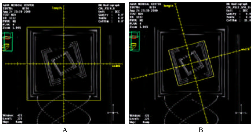
Fig. 6. The DRR and the virtual simulation images for the collimator rotation test. A) 24 × 24 cm 2 field size and 0° collimator angle, B) 12 × 12 cm 2 field size and 15° collimator angle.
