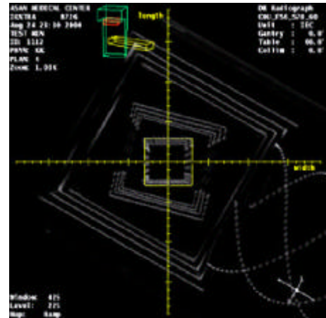
Fig. 7. The DRR and the virtual simulation images for the couch rotation test. 6 × 6 cm 2 field size and 60° Couch angle.
