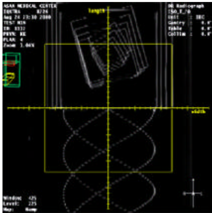
Fig. 8. The DRR and the virtual simulation images for the isocenter shift test. Couch (isocenter) was shifted 12 cm inferior. DRR images of four 24 × 24 cm 2 squares are perfectly aligned in a line.
