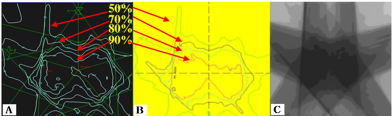
Fig. 4. Isodose comparison of the phantom plan and the film dosimetry. (A) Phantom isodose distribution generated by RTP, (B) Result of the film dosimetry, (C) Film image for phantom plan.
