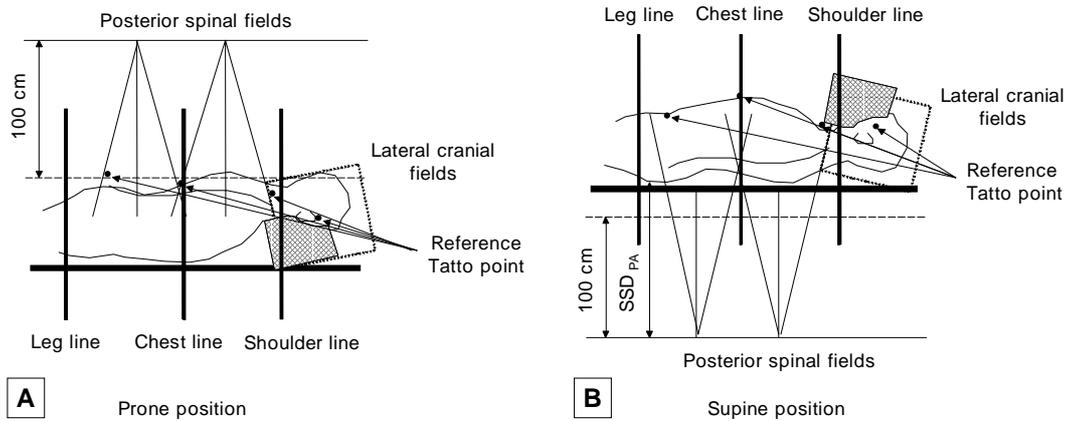
Fig. 2. Geometry of craniospinal irradiation; (A) prone position, (B) supine position. The isocentric, parallel-opposed lateral cranial fields, a posterior thoracic spine field and a posterior lumbar spine fields are schematically shown. The reference point and line is marked for the patient setup.
