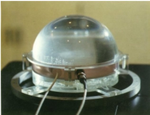
Fig. 1. A Multi-purpose phantom for stereotactic radiosurgery developed in Seoul National University Hospital (SNUH).
