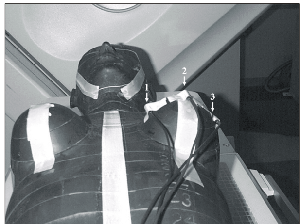
Fig. 1. Phantom and diodes setup for measurement of the doses on the contralateral breast and the breast under treatment. The directional dependence of the sensitivity of diodes was adequately considered in their setup. The diodes with the proper build thickness were calibrated to detect the dose at maximum depth for 6 MV X-rays. From the medial side toward the lateral side, the positions of the diodes are noted as positions 1, 2, and 3, consecutively.
