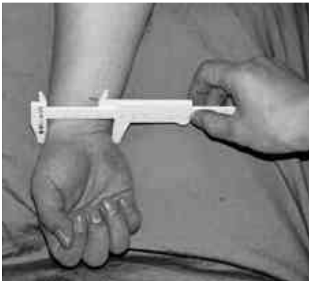
Fig. 1. Measurement Method of Wrist Depth and Width with Engineering Caliper
